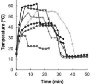
*Figure 1.* Temperature profiles obtained from commercial and domestic washing machines.
