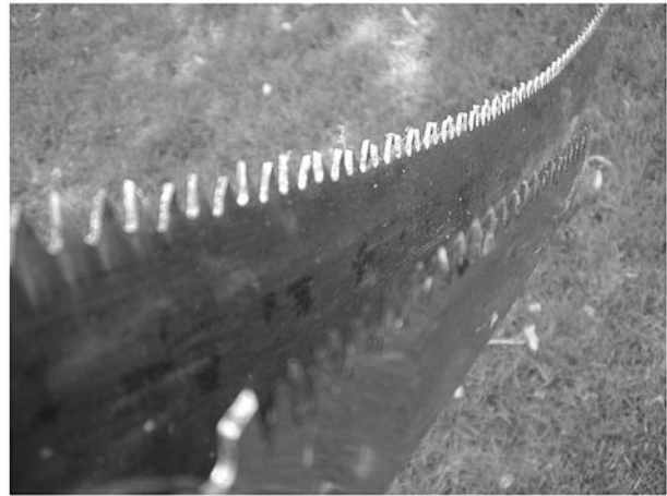
Figure 2. Newer pruning saws have little or no "set" as the back of the saw blade is thinner than the blade area. These saws also cut in either direction due to the configuration of the teeth.
