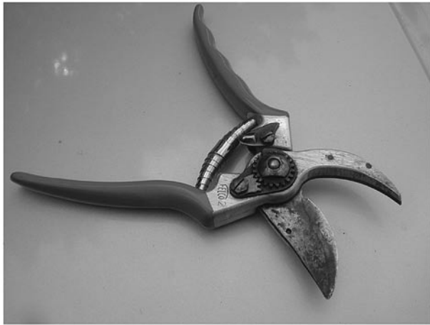
Figure 1. A hand pruner with a bypass type of cutting blade. This pruner should not be used to cut branches larger than 1/2" in diameter.
